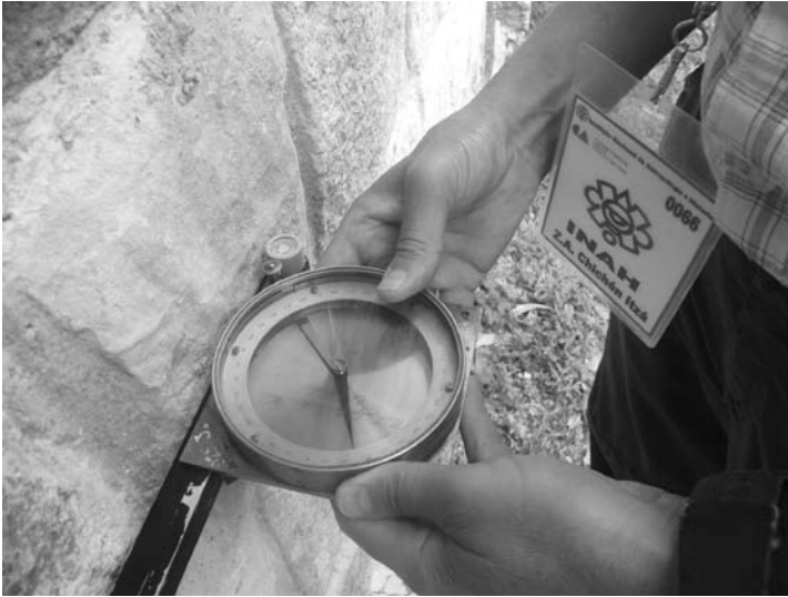
Figure 5: Measurements with precise ('mining') magnetic compass equipped with a special fitting (kindly provided by Ass. Prof. Radim Blažek, Faculty of Geodesy, TU Prague, Czech Rep.; photo © D. Lampířová, 2010).
