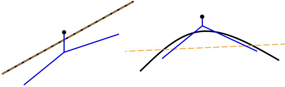
**Figure 6: Possible structural elements of the filter (blue line), actual surface (black line), trend surface (orange dashed line).**
