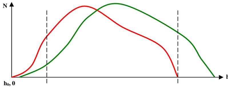
**Figure 2: Choosing the appropriate filter kernel is problematic because elevation histograms of vegetation (green line) and terrain (red line) are similar (schematic image), which can lead into errors of either first or second type. Note that the figure shows absolute heights whereas morphological filtering works on slopes.**
