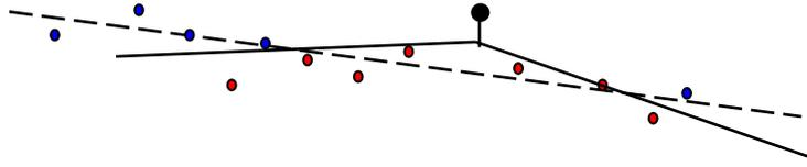
**Figure 8: Structural element of the filter; black point is rejected because of its position regarding red points.**
