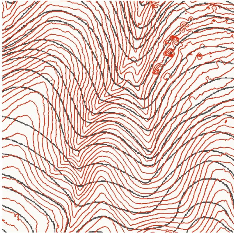
**Figure 10: The comparison between elevation contours generated with LIDAR (red) and contours from a map in the scale of 1:5000 (grey; source TTN5 2004, © Surveying and Mapping Authority of the Republic of Slovenia); LIDAR contours provide more information about the relief.**
