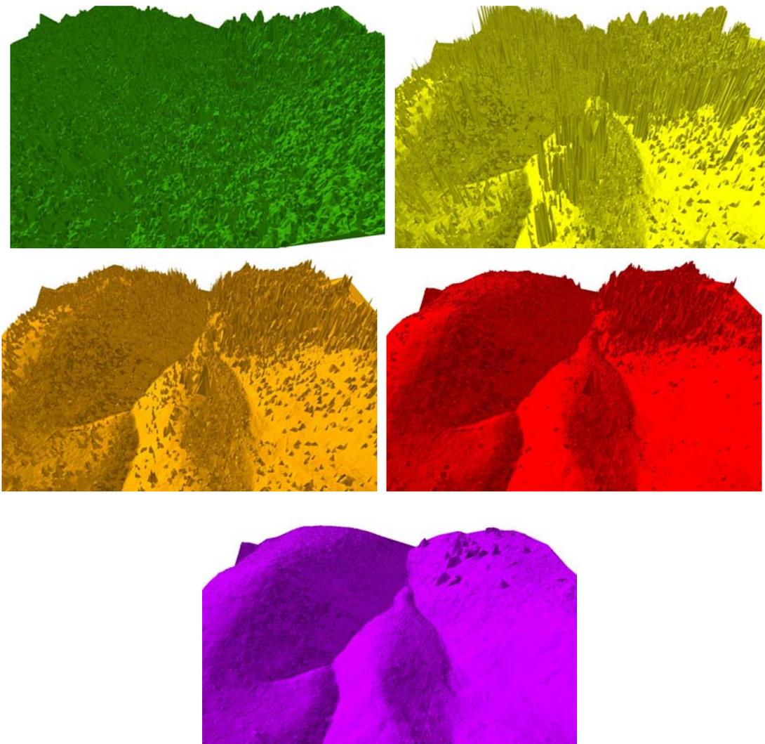
**Figure 9: The first echo data (green), the last echo data (yellow), the first step results (orange), the second step results (red), the final results (purple; some vegetation points that were not rejected can be seen on the right side).**
