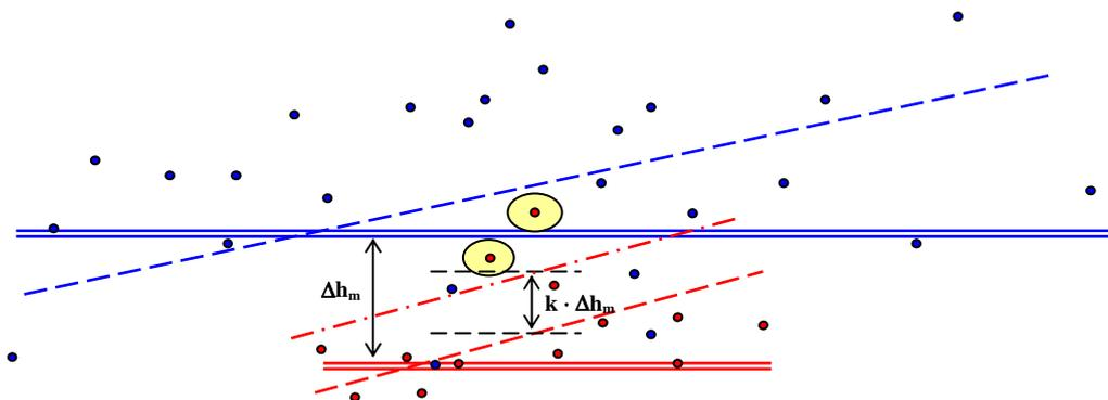
**Figure 4: Last echo points (red dots), first echo points (blue dots), red double line (horizontal surface of last echo data), blue double line (horizontal surface of first echo data), red dash line (trend surface of last echo data), blue dash line (trend surface of first echo data), red dash-dot line (threshold), dots marked with yellow are above threshold and that is why they are excluded.**
