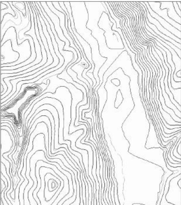
Figure 5: Computed contour lines (in black) over original vector contour lines (in gray). On the left where two sets of contours doesn't fit, it is remarkable gross error.
