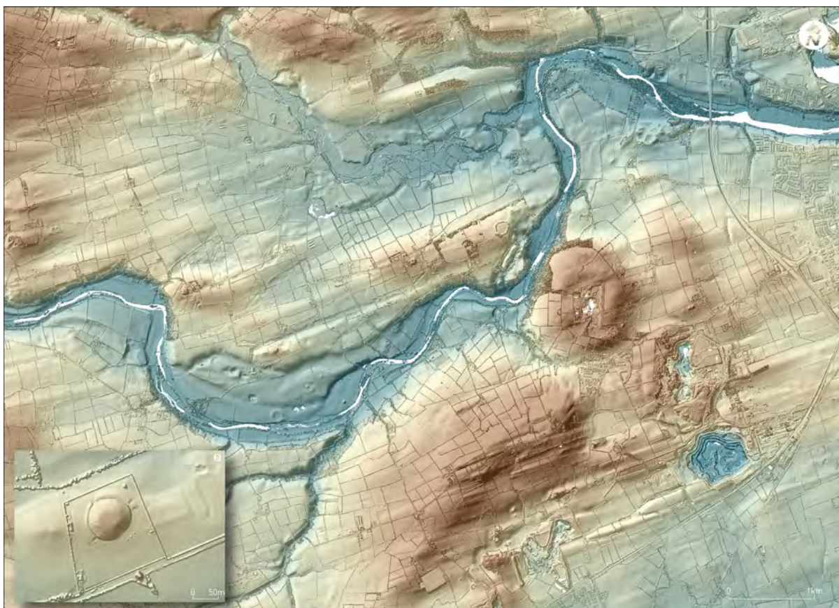
Figure 25: ALS derived DSM relief shaded model of the Brú na Bóinne landscape, enlargement around Newgrange passage tomb (Meath County Council/The Heritage Council/The Discovery Programme).
