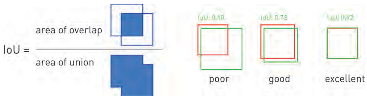
Figure 19: Illustration of Intersection-over-union (IoU) as a similarity measure for object detection on images. Image taken from Wikipedia ( https://en.wikipedia.org/wiki/Jaccard_index ).
